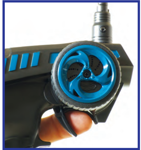
When pushed away the model should brake (and then move in reverse if applicable) if not simply flick the throttle switch to the 'Rev' position.
