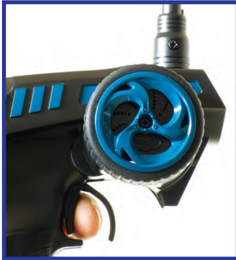
When pulled back to the handset the model should move forwards, if not flick the Throttle switch to the 'Rev' position.
